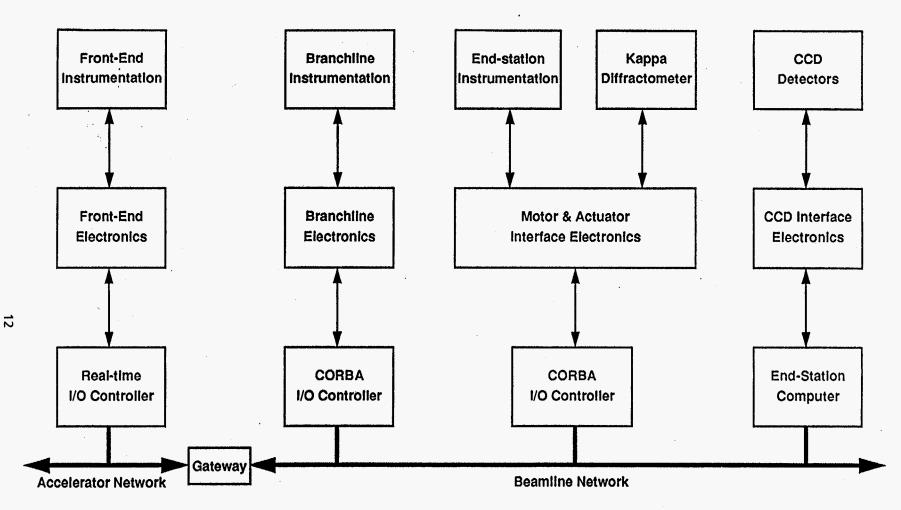
The front-end instrumentation is part of the accelerator EPICS control system which is based on the VxWorks real-time kernel and a distributed real-time database. The branchline and end-station instrumentation are controlled by distributed CORBA objects running on NeoSolaris-based SPARC computers. The CCD detector is directly interfaced to the experimenter's workstation.
