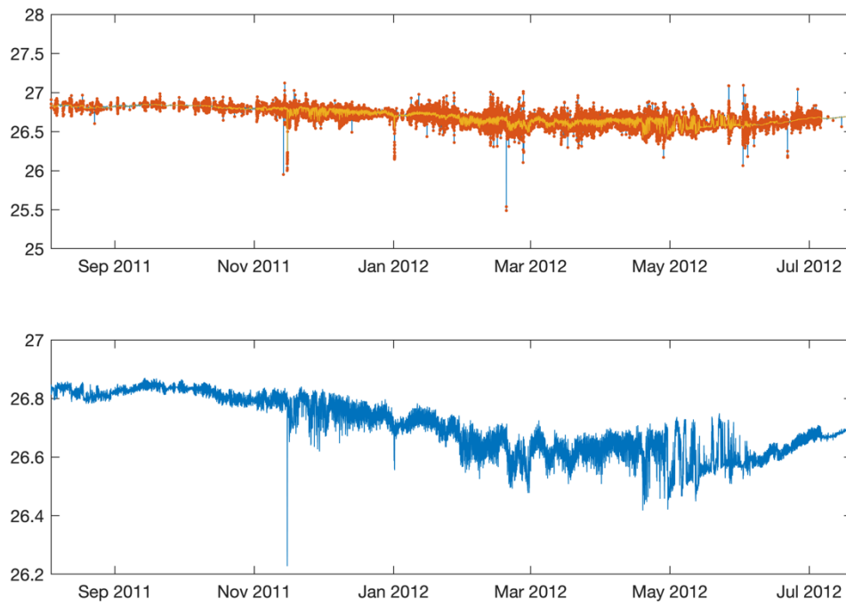
Figure 14. Potential density flagging for the SOTS Pulse-8 unpumped SBE37SM sensor at 105m. Top: thin blue line: raw temperature, orange dots: spikes based on 0.02 departure from smoothed record (yellow). Figure 8 caption has smoothing details. Bottom: Expanded view of potential density variations after removal of these spikes.
