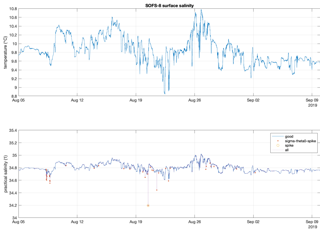
Figure 18. Salinity spikes identified from sigma-theta excursions for the SOFS-8 surface-float mounted CTD.
