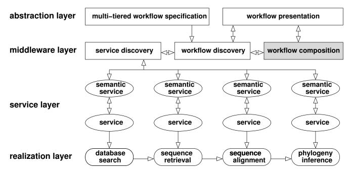
Figure 2: A four-layered architecture for workflow abstraction using Semantic Web technology.
