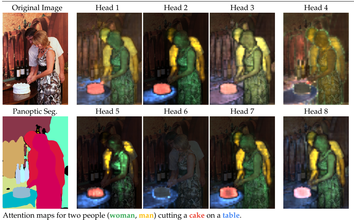
Figure C.6. Visualizing the transformer M2P attention maps for selected predicted masks. We observe that head 2, together with head 5, 7, and 8, mainly attends to the output mask regions. Head 1, 3, and 4 gather more context from broader regions, such as semantically-similar instances (scene 1 head 1) or mask boundaries (scene 2 head 4). In addition, we see that head 6 does not pay much attention to the pixel-path, except for some minor firings on the playing field and on the table. Instead, it focuses more on M2M self-attention which shares the same softmax with M2P attention (Equation (4.14)).
