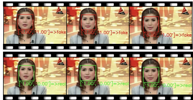
Figure 1. Adversarial Deepfakes for XceptionNet [40] detector. Top: Frames of a fake video generated by Face2Face being correctly identified as fake by the detector. Bottom: Corresponding frames of the adversarially modified fake video being classified as real by the detector.
