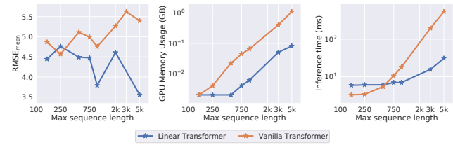
Fig. 5: Comparison of RMSE_{mean} , GPU usage, and inference time vs. driving trajectory sequence length (log-scale) for linear and vanilla Transformers over the Open-ACC dataset.
