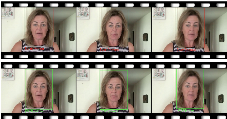
Fig. 1. Adversarial Deepfakes for an EfficientNet [65] based Deepfake detector. Top: Frames of a fake video generated by Face2Face being correctly identified as fake by the detector. Bottom: Corresponding frames of the adversarially modified fake video being classified as real by the detector.
