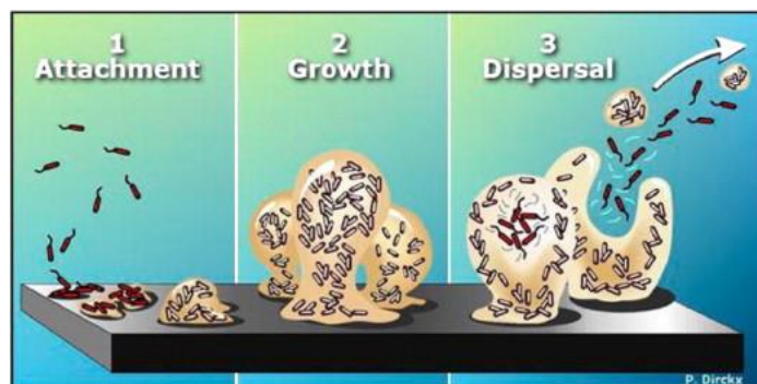
Fig. 8. Schematic illustration of biofilm formation on membrane surface (adopted from [171])
