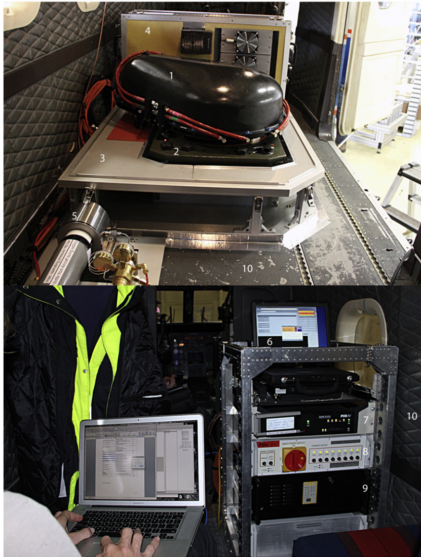
Fig. 2. Top: APEX instrument as mounted in Dornier DO-228 aircraft with N2 pressure system (bottom left), APEX on stabilizing platform (middle) and climate control (top); bottom: operator rack (right) and upload of configuration and flight data (left). Legend: 1 APEX instrument, 2 stabilizing platform, 3 interface plate, 4 thermal control unit, 5 nitrogen supply, 6 flight management computer, 7 inertial navigation system and GPS, 8 power distribution, 9 central storage unit, 10 aircraft bay. Photo: M. Jehle
