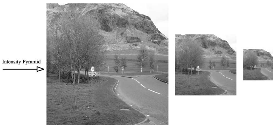
Fig. 15. The intensity pyramid built from the photograph given in Fig. 13.
