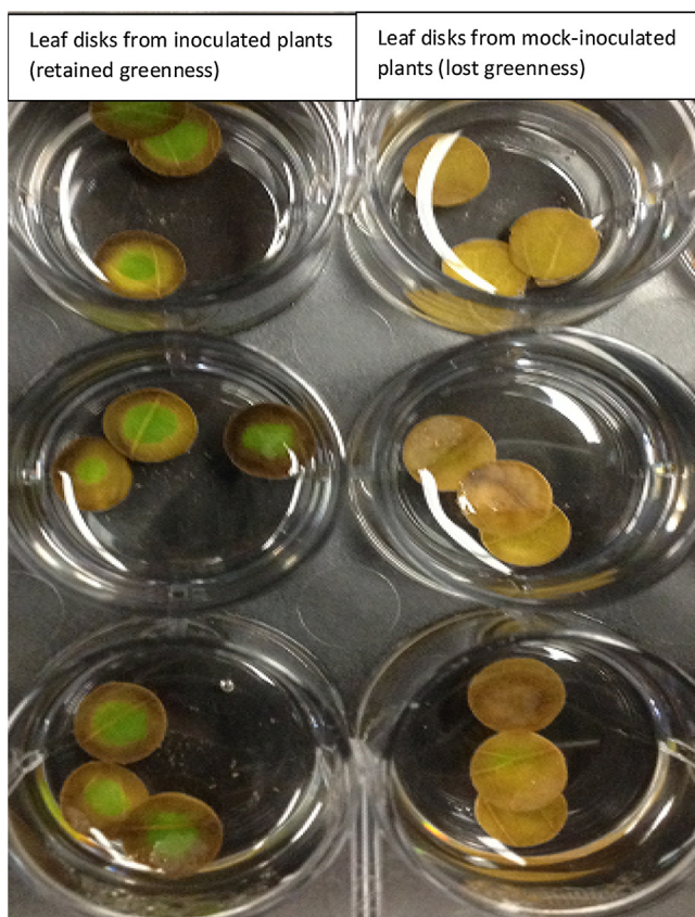
Fig. 4. Effect of inoculation on paraquat induced oxidative stress (ROS) under laboratory conditions. After 48 h of exposure to paraquat, leaves from plants that were inoculated with endophytes remained green (left) while leaves from the mock-inoculated plants were photobleached (right). Leaf disks were sampled from leaf tissues of similar size, developmental age, and location for comparison.
