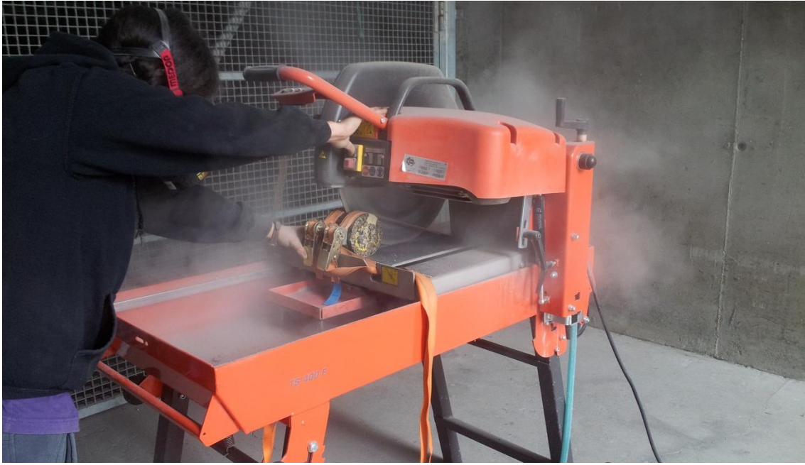
Figure 4. Cutting process of 'mother' specimens (101.6 mm high) to obtain two 'twin' specimens (50 mm high)
