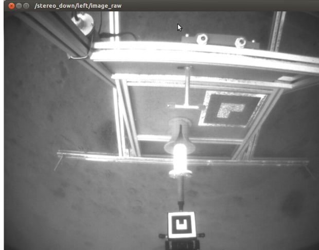
Figure 19: Plugging the connector at the Sant Feliu de Guixol harbour.
