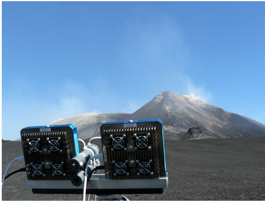
Fig. 1. Cameras imaging SO 2 emissions \approx 2 km from the summit craters of Mt. Etna. The telescopes between the cameras were incidental to the camera set up.
