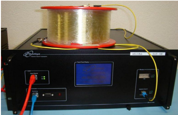
Figure 7. (a) Picture of one id Quantique device. Alice and Bob device look exactly the same. (b) Secret key rate of system id Quantique1 over one day.
