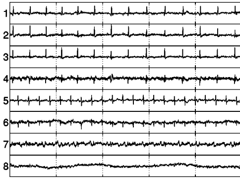
FIG. 17. Estimated independent components using JADE.
