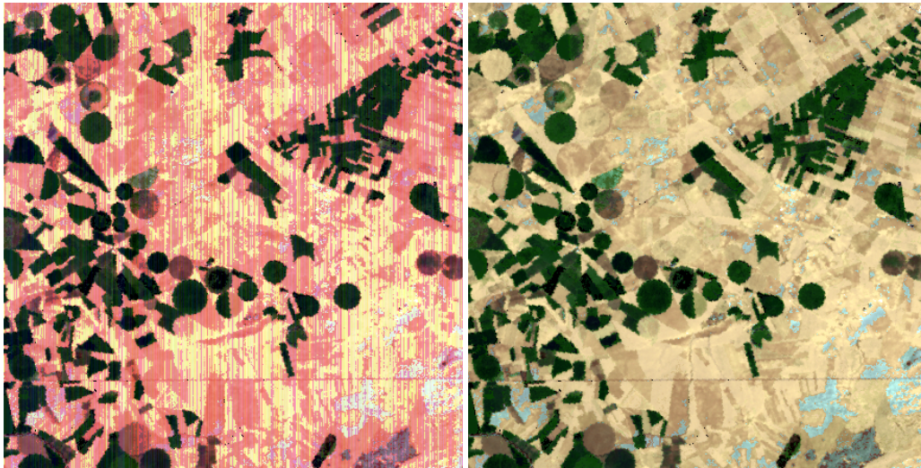
Figure 6. Red-green-blue composites from a simulated EnMAP dataset over Barrax (Spain) illustrating the conversion from digital numbers ( left ) to radiometrically-calibrated radiance data ( right ). The switch between high and low radiometric gain modes is visible in the digital number image as yellowish and pinkish patches.
