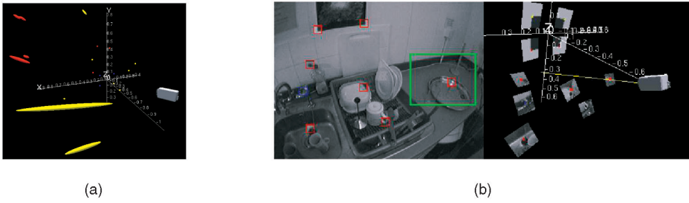
Fig. 1. (a) A snapshot of the probabilistic 3D map, showing camera position estimate and feature position uncertainty ellipsoids. In this, and other figures, in the paper the feature color code is as follows: red = successfully measured, blue = attempted but failed measurement, and yellow = not selected for measurement on this step. (b) Visually salient feature patches detected to serve as visual landmarks and the 3D planar regions deduced by back-projection to their estimated world locations. These planar regions are projected into future estimated camera positions to predict patch appearance from new viewpoints.
