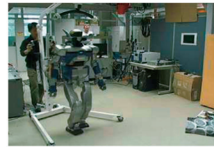
Fig. 9. HRP-2 walking in a circle. The robot is walking autonomously and tether-free with SLAM processing on-board and a wireless Ethernet link to a control workstation. The support cradle seen is only for safety purposes.
