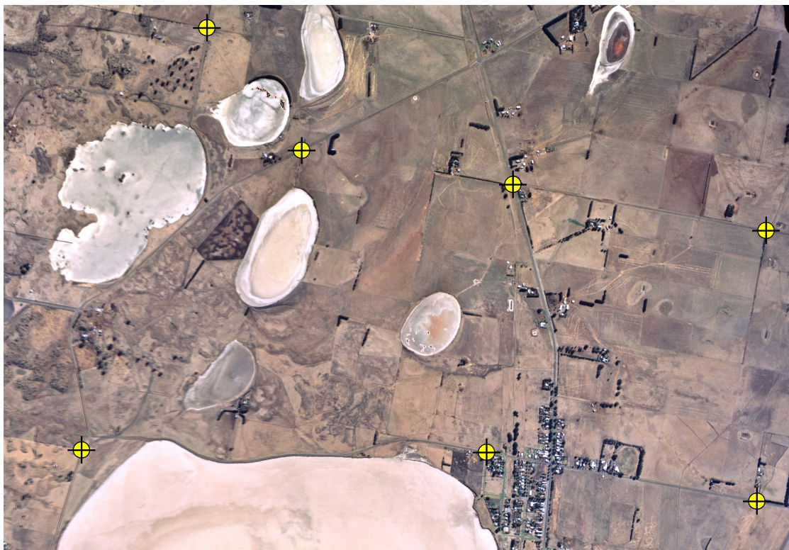
Figure 2. An example of scanned natural colour aerial photographs with highlighted positions of GCPs measurements.
