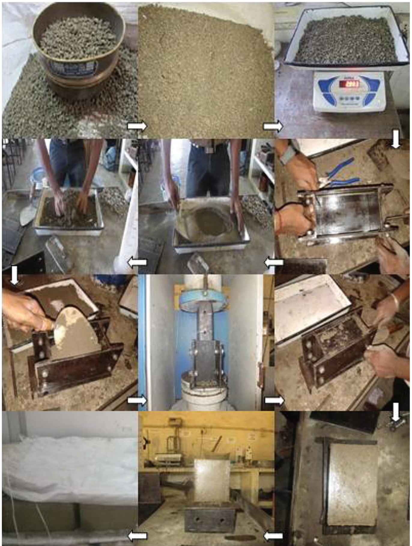
Fig. 4: Graphic description of the casting and curing of stabilized earth blocks
