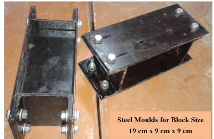
Fig. 3: Steel moulds adopted for the moulding of stabilized blocks
