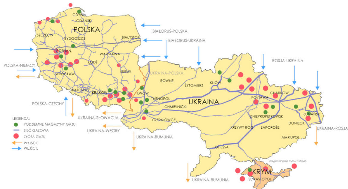
Fig. 1. Poland and Ukraine with transfer infrastructure, underground gas storage (UGS) facilities and earth gas reservoirs. Source: own elaboration based on www.naftogaz-europe.com and http://www.pgnig.pl/ (accessed on 30 April 2018)
