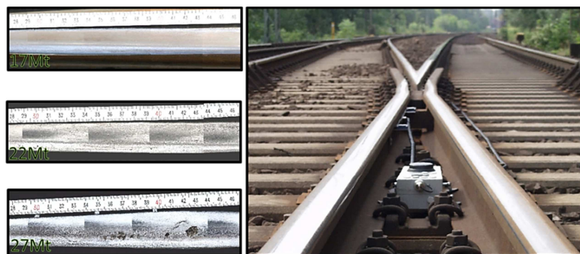
Fig. 1: The track-side inertial measurement systems: left – RCF development images and their times in megatons (Mt), right – ESAH-M [17]).
