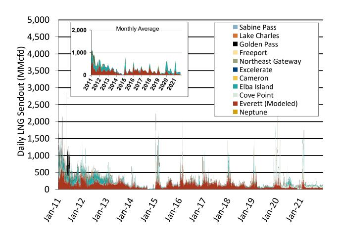
Notes: Everett data includes flows onto the AGT and TGP interstate lines, plus estimates of flows to the Mystic 7 power plant, Keyspan Boston Gas, and LNG trucked out of the terminal. Excludes flows to the Freeport LNG which flows via intrastate pipelines.
