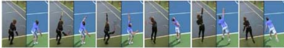
(a) Full body motion reconstruction using a small number of cheap accelerometers, from [3]. Motion is synthesized by using low-dimensional signals from wearable accelerometers to index into a motion graph created using optical motion capture.
