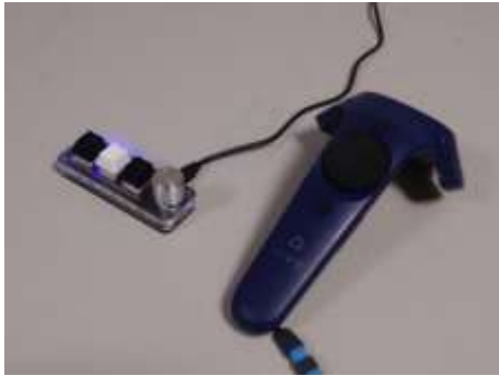
Figure 3: The left-hand-operated device and a VIVE controller used in the experiment
