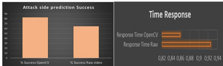
Fig. 3. Time response (seconds) and attack (side from it is launched) guessing success (%) (obtained from [31])
