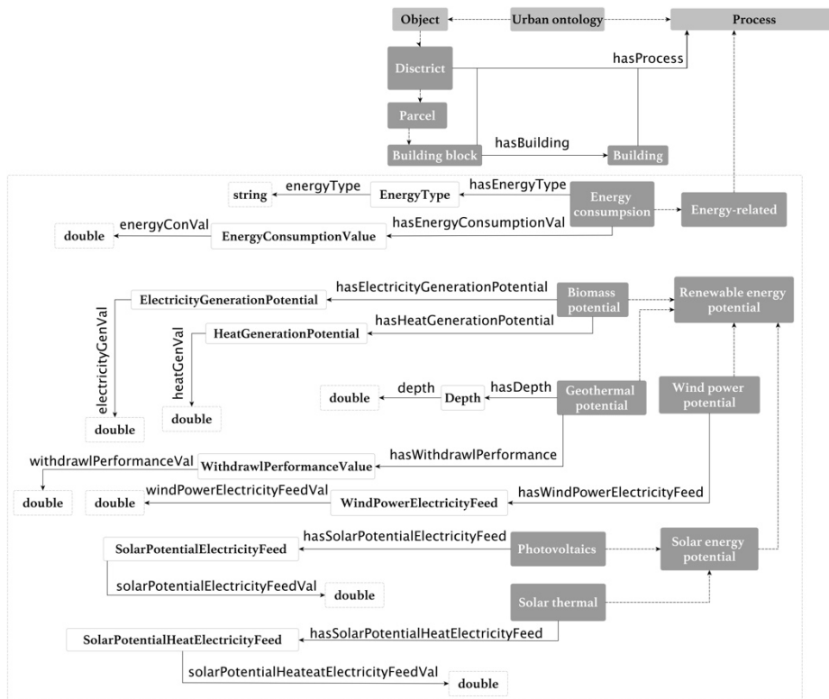
Fig. 4. Energy-related processes in the surrounding environment
