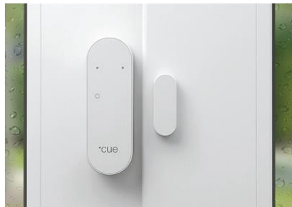
Fig. 6. Develco Door/Windows sensor
