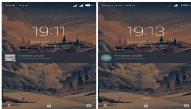
Fig. 5. Airtel service before and after the Jammer was “ON”.
