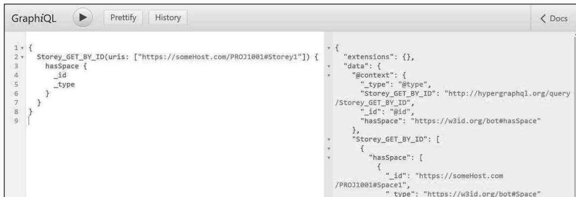
Figure 2: HyperGraphQL query to retrieve the instances of bot:Space of one specific instance of bot:Storey, by using Storey_GET_BY_ID.
