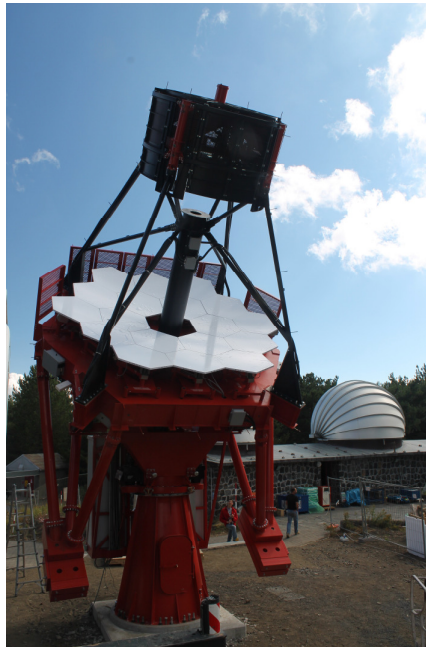
Figure 1. ASTRI telescope prototype ready to start System verification
