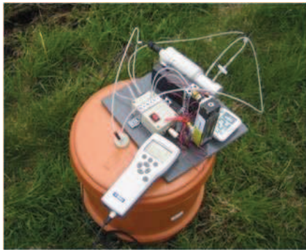
Fig. 1. Chamber and Vaisala GMP 343 for CO 2 measurements
