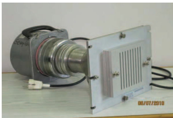
Fig. 3. The set-up of High Volume 20CFM Cascade Impactor (Staplex, Andersen)
