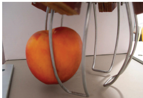
Fig. 6. The fingertip geometry is much larger than the fruit size.
