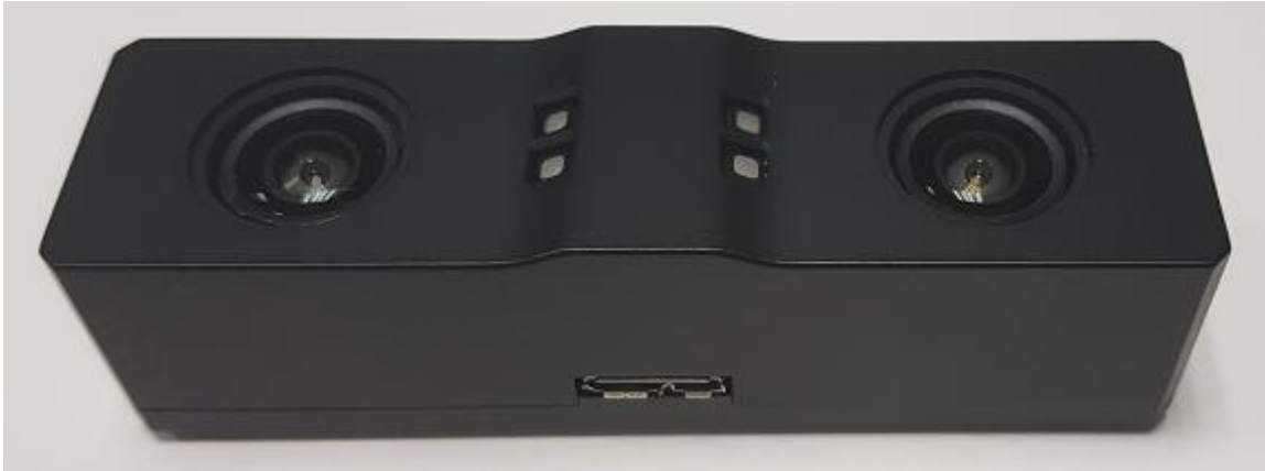
Figure 1. eAP87606D100 - 6cm baseline with IR illumination
