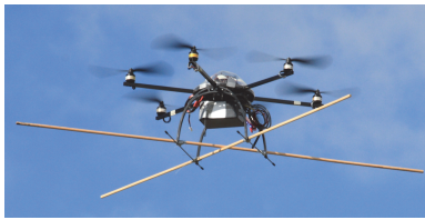
Figure 3: The “Hexacopter” UAVs used in the flight tests presented in Section 5.
