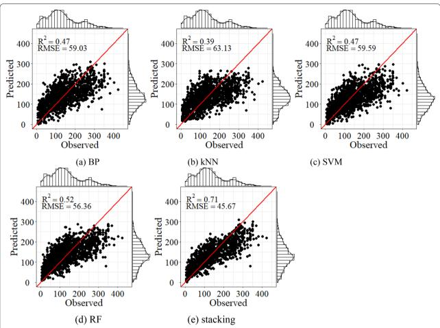
Fig. 8 Scatter plots of the observed AGB against the predicted values by **a** BP, **b** kNN, **c** SVM, **d** RF and **e** stacking using the spectral variables and LiDAR variables extracted from ICESat-2 (Mg/ha)
