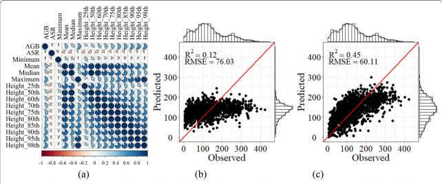
**Fig. 10** a Correlation coefficient matrix of LiDAR variables and AGB, and scatter plots of the observed AGB against the predicted values by linear regression using **b** the spectral variables, and **c** spectral variables and LiDAR variables (Mg/ha)
