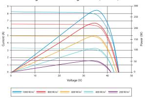
Excellent performance under weak light conditions: at an irradiation intensity of 200 W/m $^2$  (AM 1.5, 25 °C), 95.5% or higher of the STC efficiency (1000 W/m $^2$ ) is achieved
