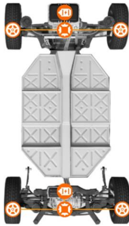
Fig. 4. Schematic representation of the Tograc qE's powertrain simulation in BeamNG. The mathematical model of individual components can be further subdivided but have been omitted in favor of simplicity. This diagram shows that it's also possible to include two different power sources into the powertrain simulation. The two powertrain trees each consist of an electric motor that is connected to a differential, which is connected to the front/back wheels.
