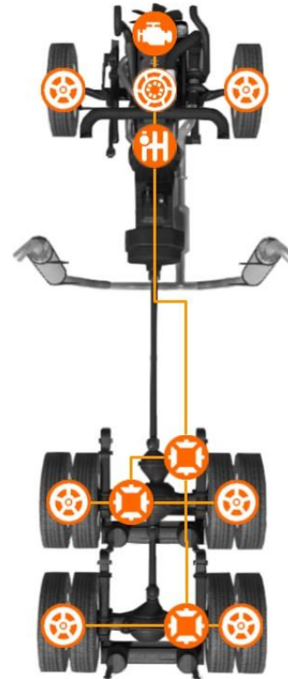
Fig. 3. Schematic representation of the powertrain simulation of the Gravid T65 in BeamNG. The mathematical model of individual components can be further subdivided but have been omitted in favor of simplicity. The individual components of the powertrain are, from top to bottom and as they are connected: engine, clutch, gearbox, first differential that distributes the power between the two-wheel pairs and the consecutive differential that distributes the power within the individual wheel pairs.
