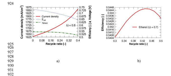
Figure 11. Effect of recycling on a SOFC plant fed by ethanol, a)  $U_f = 0.8$  and b)  $U_f = 0.7$ .
