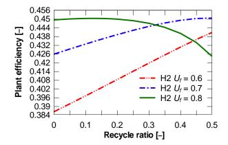
Figure 8. Effect SOFC fuel utilization factor on plant efficiency, fed by hydrogen.
