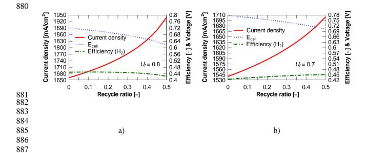
Figure 7. Effect of recycling on a SOFC plant fed by hydrogen, a)  $U_f = 0.8$  and b)  $U_f = 0.7$ .
