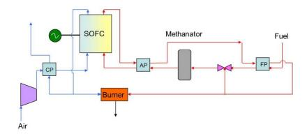
Figure 10. Plant design fed by methanol, ethanol and DME.
