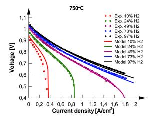
Figure 3. Cell voltage versus current density and a comparison between the modelling results and experimental data at 750°C with different fuel compositions.
