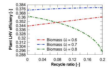
Figure 16. Effect of recycling on a SOFC plant fed by biogas from biomass gasification, a)  $U_f = 0.8$  and b)  $U_f = 0.6$ .
