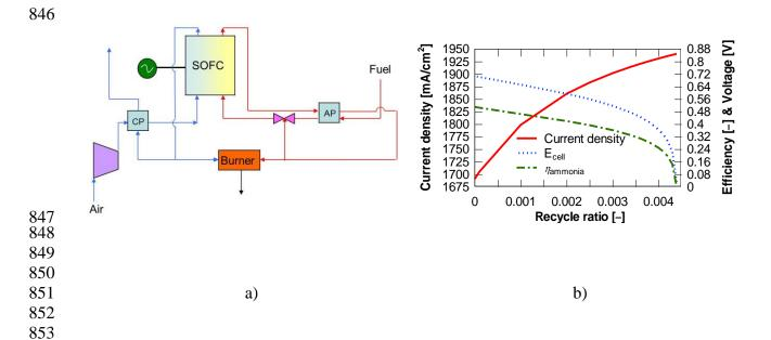
Figure 4. a) SOFC plant design fed by ammonia and b) effect of recycle ratio.
