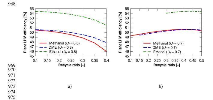
Figure 14. Effect of recycling on a SOFC plant fed by methanol, ethanol and DME, a)  $U_f = 0.8$  and b)  $U_f = 0.7$
