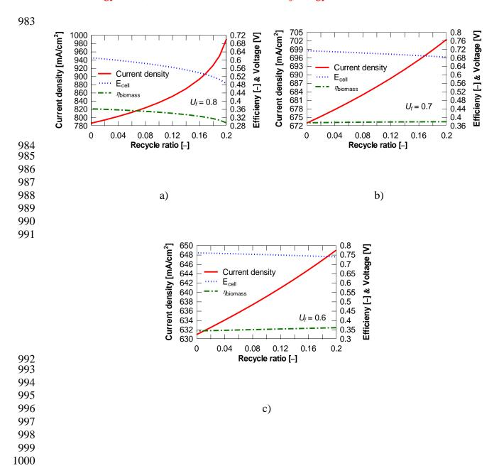
Figure 15. Effect of recycling on a SOFC plant fed by biogas from biomass gasification , a)  $U_f = 0.8$ , b)  $U_f = 0.7$  and c)  $U_f = 0.6$ .
