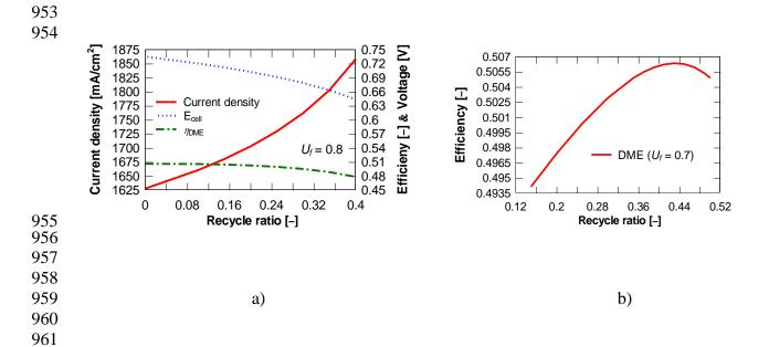
Figure 13. Effect of recycling on a SOFC plant fed by DME, a)  $U_f = 0.8$  and b)  $U_f = 0.7$ .
