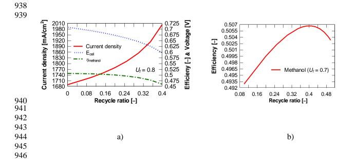
Figure 12. Effect of recycling on a SOFC plant fed by methanol, a)  $U_f = 0.8$  and b)  $U_f = 0.7$ .
