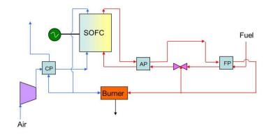
Figure 6. Plant design fed by hydrogen, alternative design.
