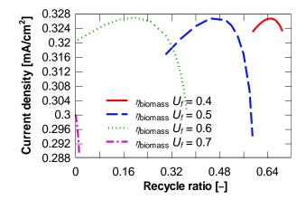
Figure 17. Effect of recycling on a SOFC plant fed by biogas from biomass gasification when number of stacks is 8.
