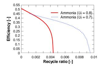
Figure 5. Effect SOFC fuel utilization factor on plant efficiency, fed by ammonia.
