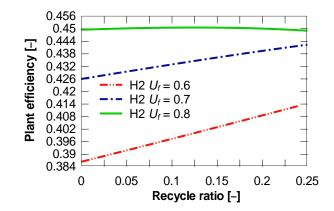
Figure 9. Effect of anode recycle for alternative plant design for hydrogen.
