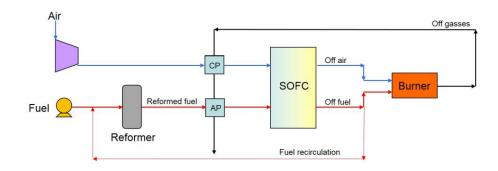
Figure 1. General fuel cell plant with anode off-fuel recirculation. CP: Cathode Preheater, AP: Anode Preheater.
