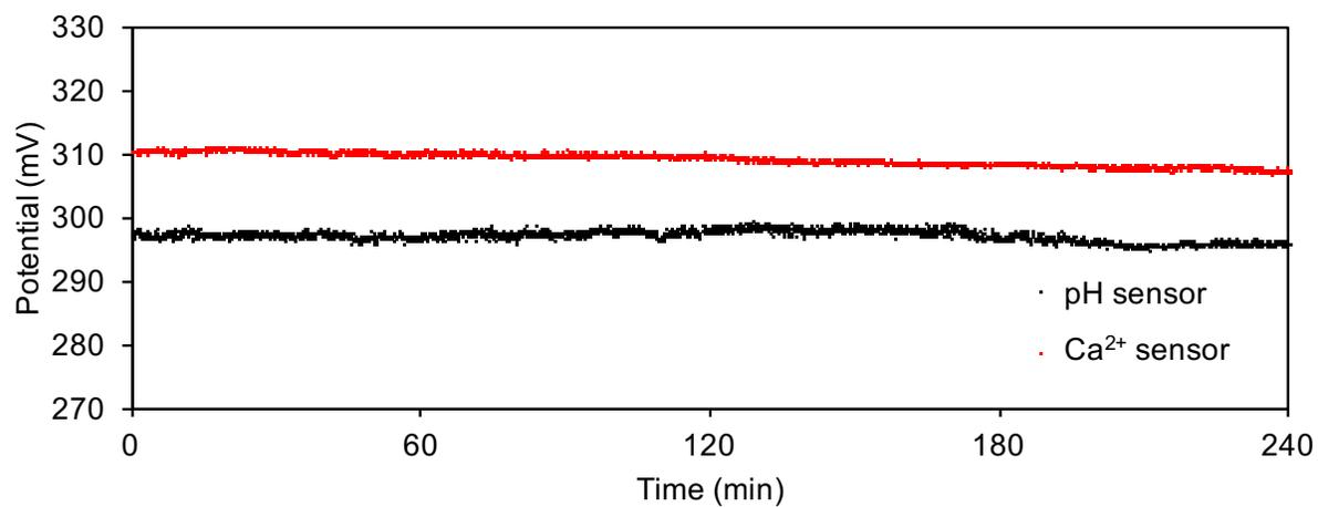
Figure S1. Long-term stability of Ca<sup>2+</sup> and pH sensors in 0.01 M acetate buffer containing 1 mM CaCl<sub>2</sub> in 4 hours. Potential is reported with respect to a standard Ag/AgCl reference electrode.
