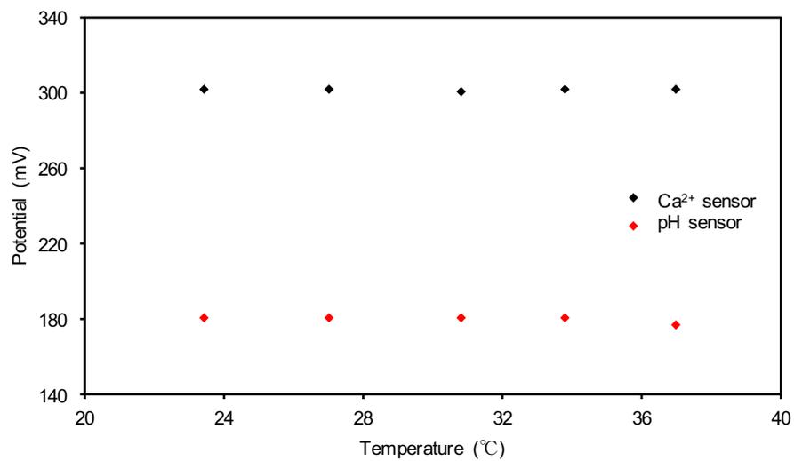
Figure S3. Temperature dependence of Ca<sup>2+</sup> and pH sensor in a solution containing 0.5 mM Ca<sup>2+</sup> in McIlvaine's buffer of pH 5.0.
