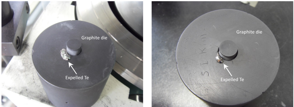
Figure S3. Pictures after transient liquid flow compacting process (spark plasma sintering) for 25 wt% Te excess \text{Bi}_{0.5}\text{Sb}_{1.5}\text{Te}_3 (Te-MS) material.
