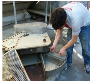
Figure 6: Eccentric weights oscillate Millikan Library, demonstrating that CSN hardware can observe resonant frequencies in buildings.
