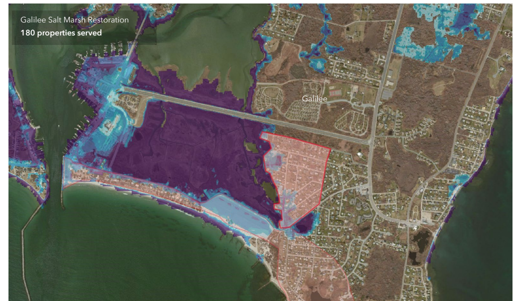
Area of protection 0.5 1 2 3+ ft Depth of flooding for a simulated 1 in 100 flood event in 2020
