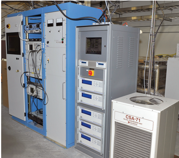
FIGURE 9. The gyro-TWT high-voltage supply and system electronics. The helium compressor at the right forms half the cryocooler, along with the cold head mounted in the magnet cryostat seen in Figure 5.
