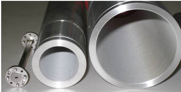
FIGURE 6. On the left is the W-band single-mode rectangular waveguide WR-10 ( TE_{01} mode). Center and right are the 1.25-inch- and 2.5-inch-diameter corrugated waveguides ( HE_{11} mode).
