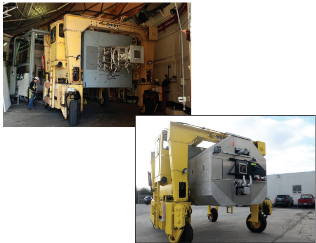
FIGURE 6. The protruding X-band feed is clearly visible in the preupgrade LRIR RF box sitting in the special transporter (above top). An octagonal extension was added to the RF box to house the W-band radar feed, duplexer, and receiver, and radio-astronomy instrumentation—K-band, Q-band, and, in the future, W-band radiometers (right). The HUSIR RF box is shown in the transporter (above bottom).
