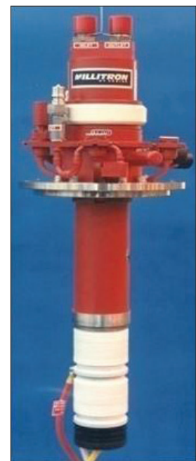
FIGURE 3. MMW required a high-power, high-frequency traveling-wave-tube amplifier. VTA-5700 tubes, similar to the one shown, were used from 1983 to 1991.
