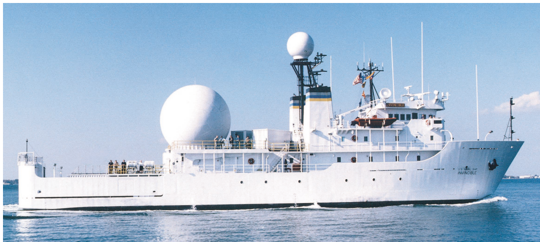
FIGURE 8. The Cobra Gemini radar (large radome) in its sea-based configuration on the Invincible , a U.S. Naval T-AGOS ship. A transportable sensor such as Cobra Gemini is designed to assist in the detection and discrimination of tactical theater ballistic missiles.
