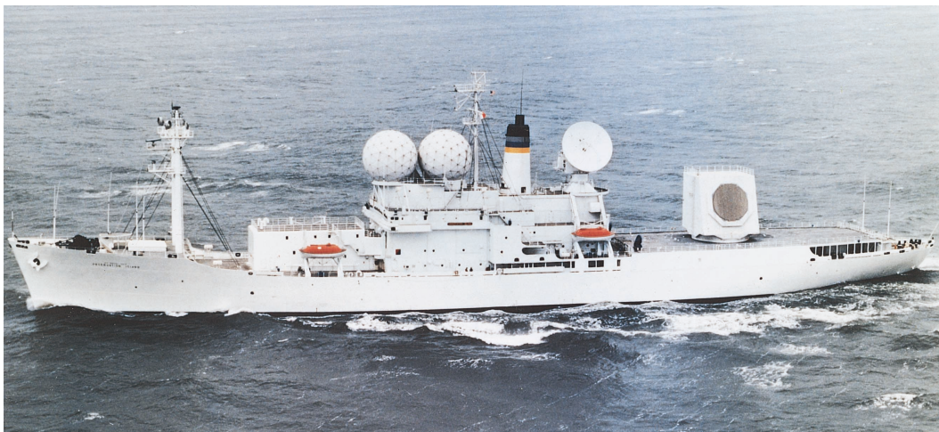
FIGURE 7. The wideband phased-array Cobra Judy radar on the U.S. Naval ship Observation Island . The S-band phased-array radar is at the stern of the ship; the mechanically scanned dish just forward of it is the X-band radar antenna. The Cobra Judy is the world's largest mobile phased-array sensor.
