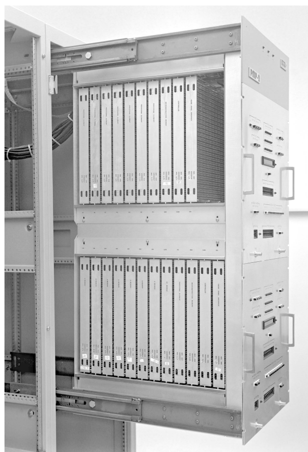
FIGURE 16. The parallel microprogrammed processor (PMP) built by Stein Associates and installed at the Burlington, Vermont, airport in 1978. This detector was displayed to visiting air traffic controllers from all over the United States, who were positively impressed with its performance.
