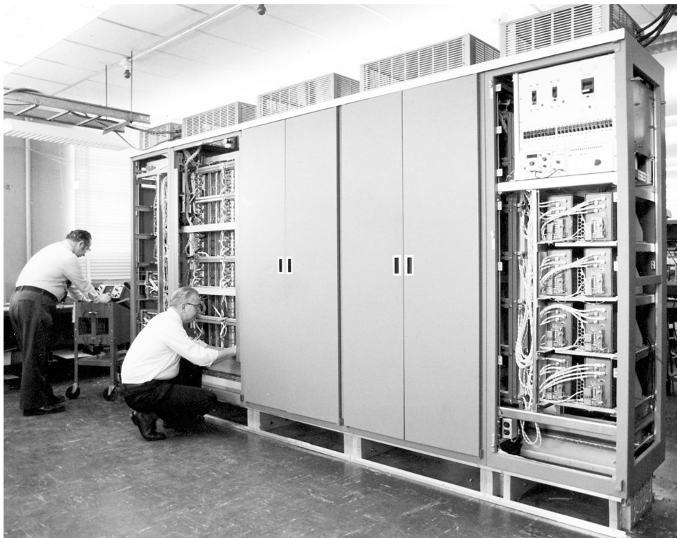
FIGURE 13. The DCS in 1979. At that time it was the fastest and largest pipelined FFT processor ever built. The system was large; it was comparable to the ALCOR all-range processor shown in Figure 3, but with an order-of-magnitude improvement in performance.
