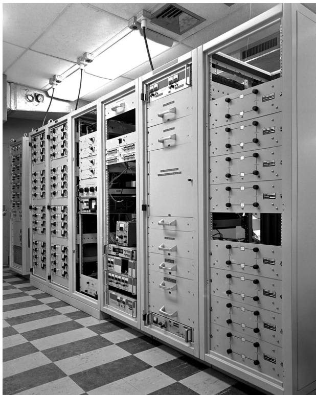
FIGURE 3. The ALCOR all-range wideband analog pulse compressor developed jointly by Lincoln Laboratory and Hazeltine Laboratory.
