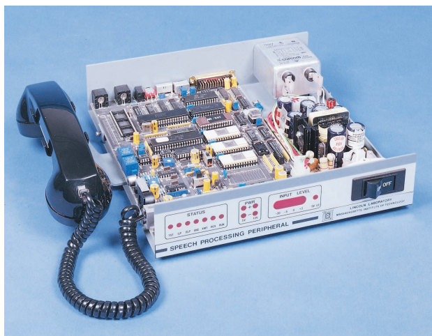
FIGURE 9. The first stand-alone compact linear predictive speech coder, or LPC vocoder, which served as a major driver and motivating force for the next-generation commercial secure telephone units (STU-III) introduced into government service during the early 1980s. This vocoder was based on the state-of-the-art commercial single-chip digital-signal-processing microcomputers available at that time.
