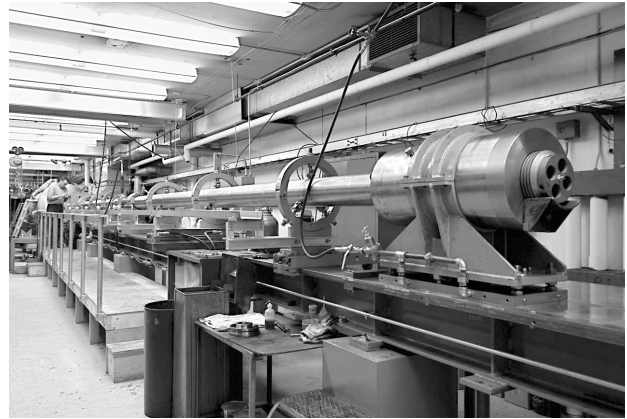
FIGURE 4. The light-gas gun used to fire pellets at ICBM velocities. This gun routinely achieved pellet velocities of over 20,000 ft/sec. On one occasion a hydrogen leak caused a pellet to be fired at 32,000 ft/sec.
