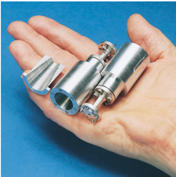
FIGURE 19. The scalar, or ridged, horns used for the 95-GHz radar. This small horn launches an almost perfect Gaussian beam that, with a properly designed optical system, provides excellent illumination of the 13.7-m primary reflector. The system provides higher power capability, broader bandwidth, lower losses, and better antenna patterns than a conventional waveguide system could at shorter wavelengths.
