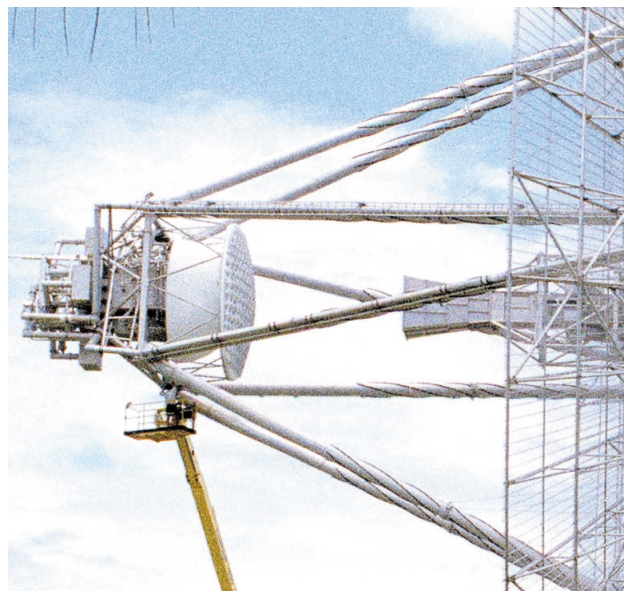
FIGURE 15. The VHF and UHF feeds of the ALTAIR radar. The white "teacup" (notice its size relative to that of the man standing below it) is the cover of the conventional five-horn focal-point feed of the VHF system. The "saucer" is the dichroic secondary reflector of the UHF Cassegrainian system with a multimode horn at the vertex. The reflector is composed of two layers of crossed dipoles that are resonant at UHF, making it an excellent reflector at UHF and almost transparent at VHF. The system angle-tracks at both frequencies, and either frequency can drive the antenna-servo system. (A similar frequency-selective subreflector was installed on the Millstone Hill radar; see the article by Stone and Banner in this issue.)
