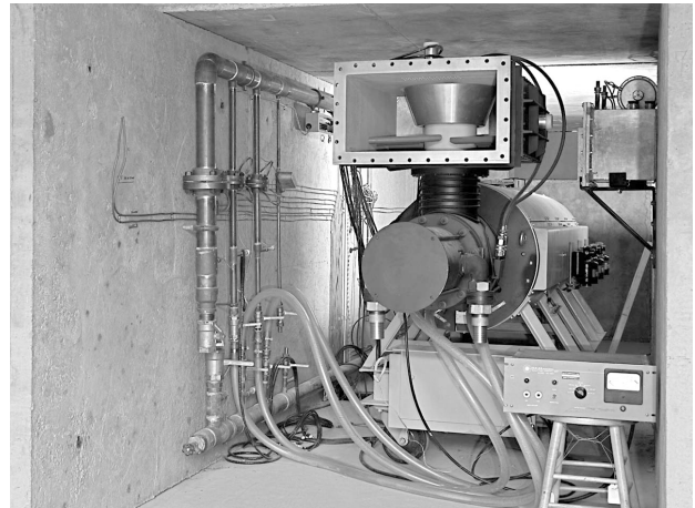
FIGURE 9. A UHF klystron designed for horizontal operation at 60-MW peak power is shown in the RTRF test stand. The heavy concrete walls provided necessary shielding against the intense X-rays generated by these tubes.
